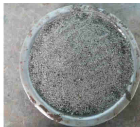
River sand and LD slag used as fine aggregate in concrete
