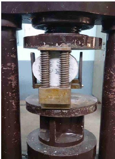
Testing of cubes & cylinder for compression and split tensile strength
